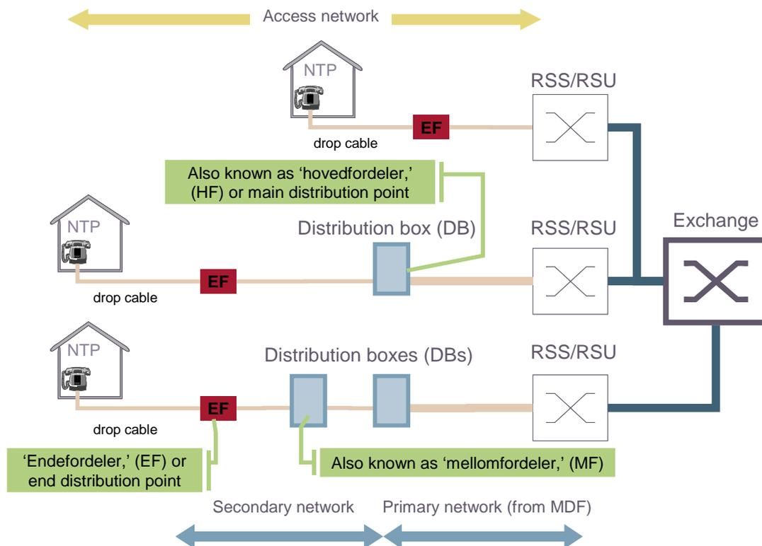
Figure 5.1: Topology of the copper access network [Source: Telenor, Analysys Mason]
