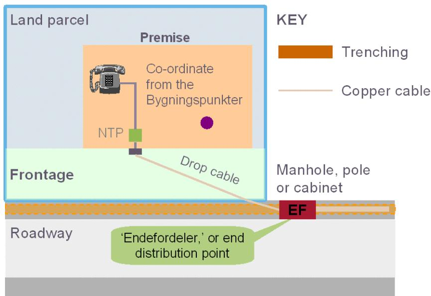
Figure 5.5: Final drop topology [Source: Telenor, Analysys Mason]
