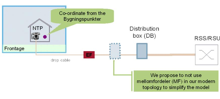
Figure 5.6: Proposed current network deployment [Source: Telenor, Analysys Mason]
