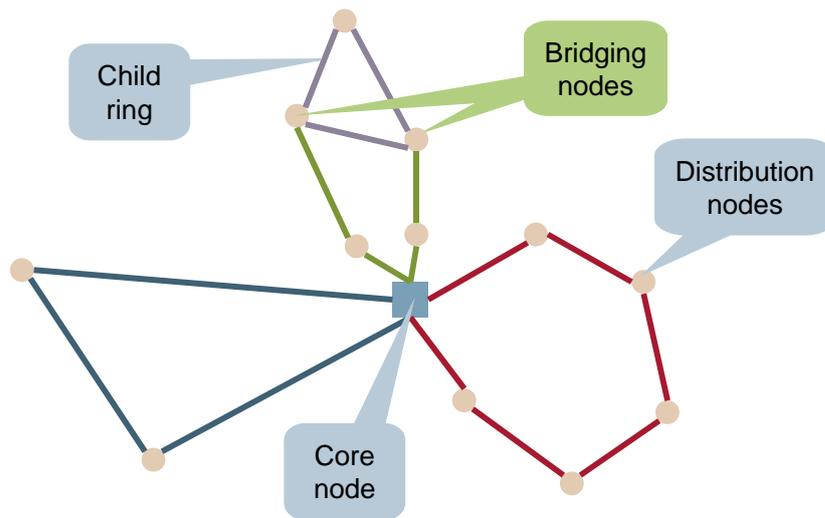
Figure A.1: Ring structures in the core network, joining distribution nodes to a core node in a set of resilient rings [Source: Analysys Mason]
