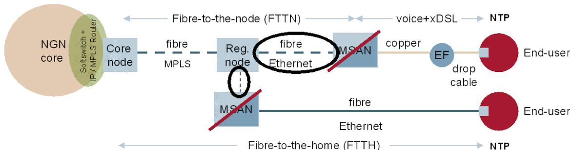
Figure 5.13: Boundary between the NG core and access network (red line) [Source: Analysys Mason]
