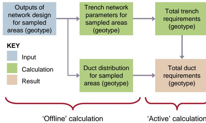
Figure 5.11: Calculation of total access network duct requirements
