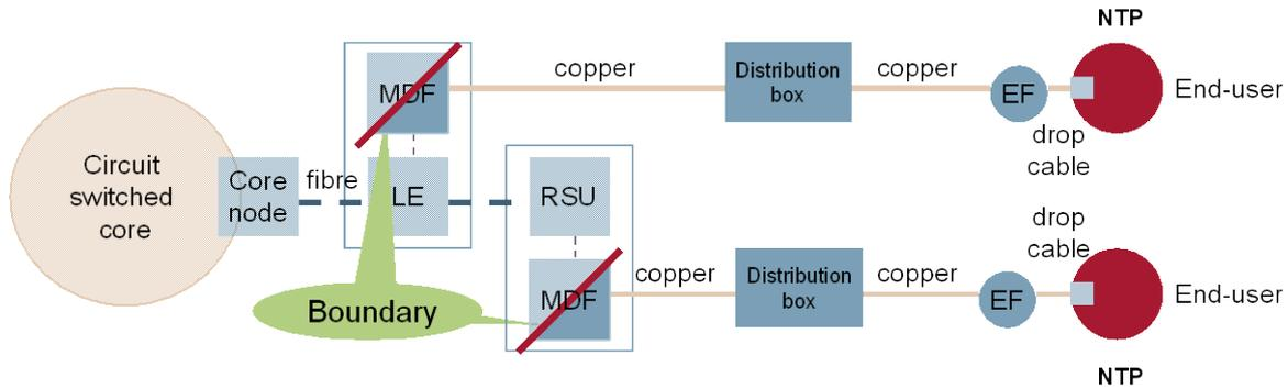
Figure 5.12: Boundary between legacy core and access network (red line) [Source: Analysys Mason]
