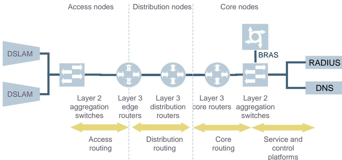
Figure 5.18: Current data core network deployment in Norway [Source: Analysys Mason]
