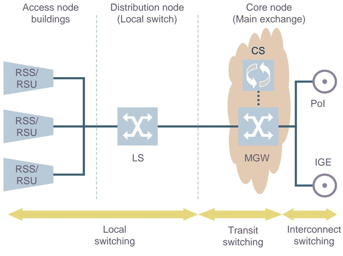
Figure 5.16: Current voice core network deployment in Norway [Source: Analysys Mason]
