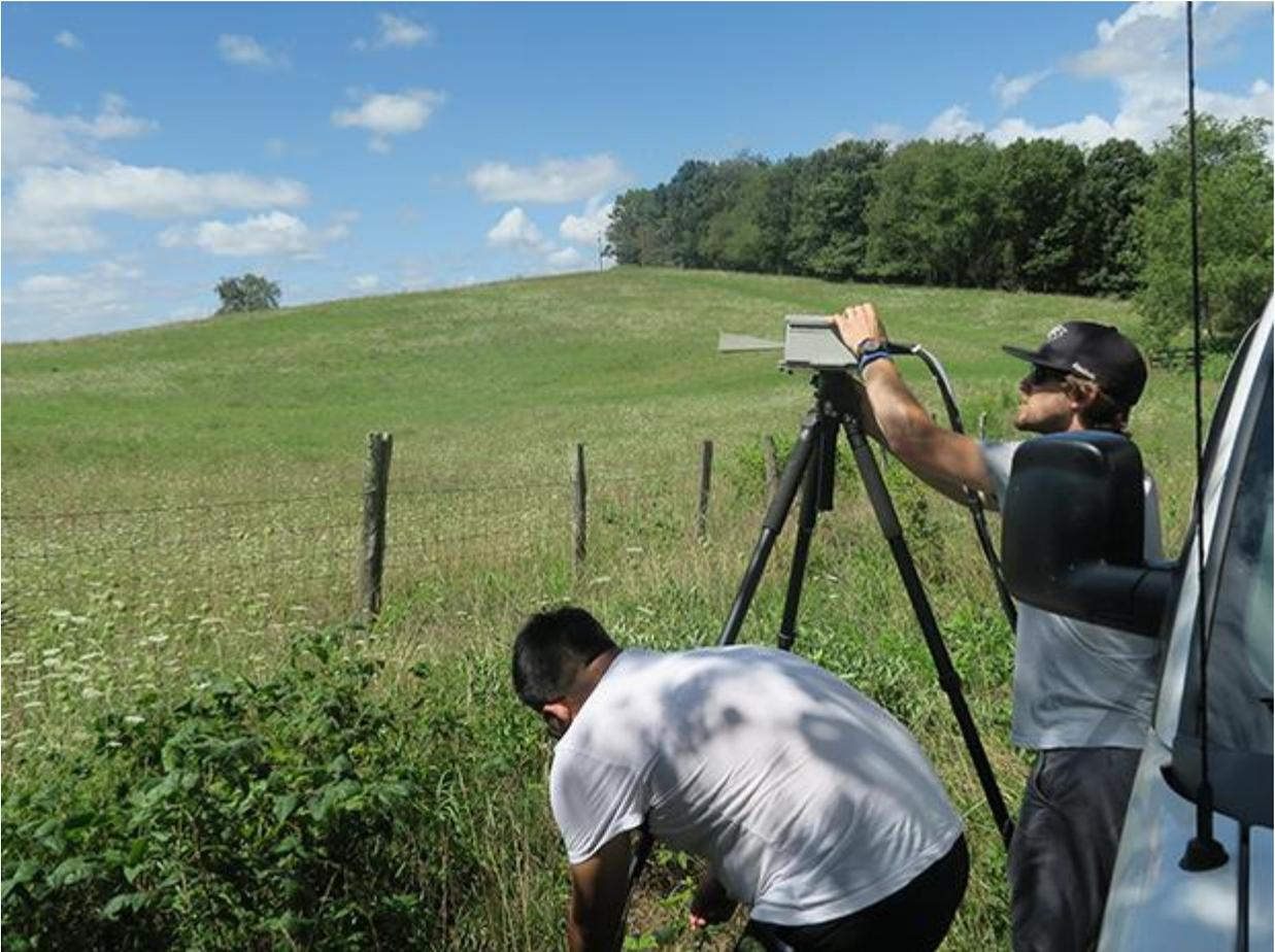
Photo: Hangsong Yan Yunchou Xing (left) and George MacCartney (right) adjust the horn antenna of their receiver to find the strongest signal during a millimeter wave measurement campaign in August. They are within line of sight of a transmitter stationed 4.3 kilometers away at the home of their NYU professor, Ted Rappaport.
