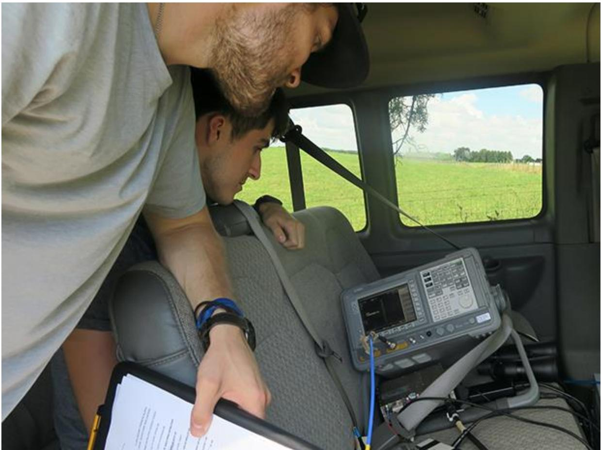
Photo: Hangsong Yan George MacCartney (left) and Jeton Koka (right) observe the signal strength from their receiver on a Keysight E4407B spectrum analyzer before recording a measurement.
